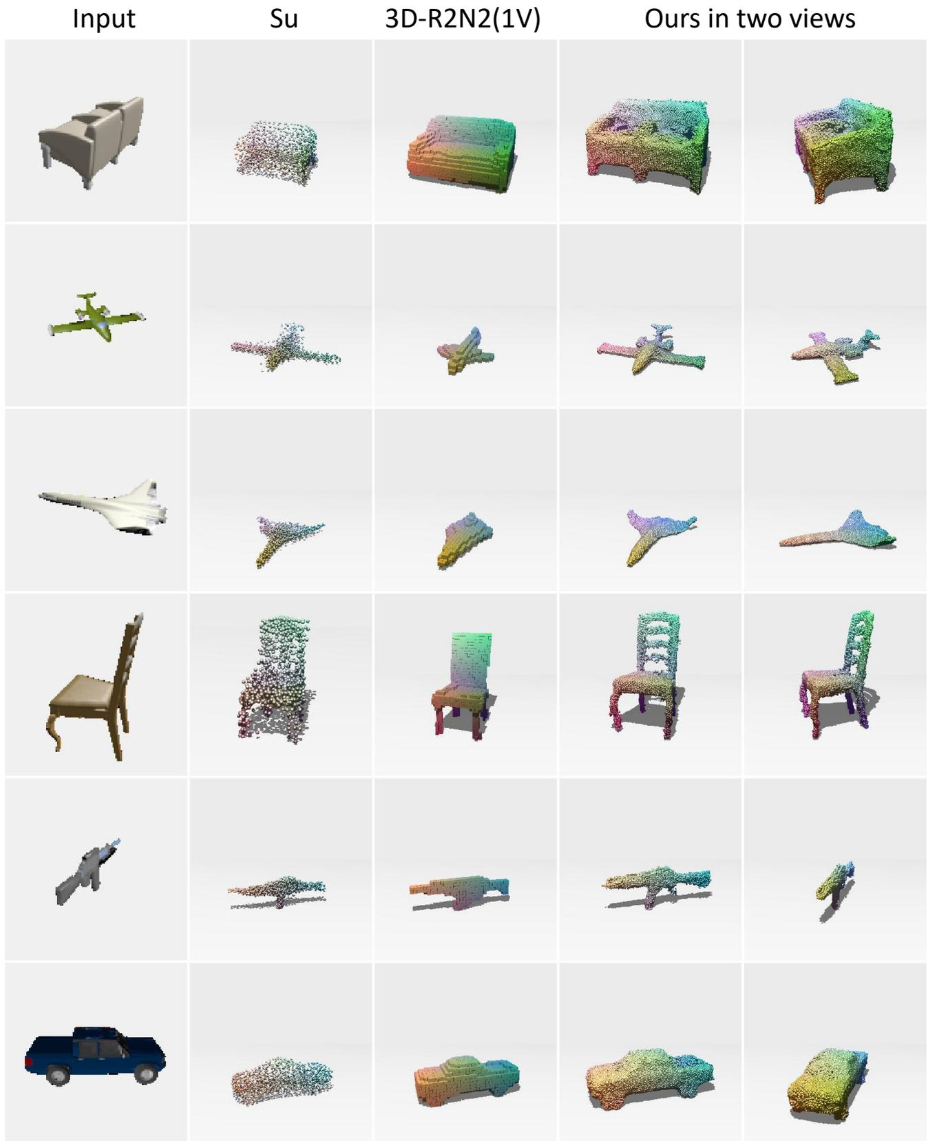
Figure F: More qualitative reconstruction results compared to Su(Fan, Su, and Guibas 2017) and 3D-R2N2(Choy et al. 2016). Note that for 3D-R2N2, we take a single input image for fair comparison. The rightmost two columns show our generated models in two views. Our results preserve more details and recover concave structures well.
