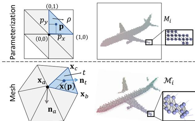
Figure A: Parameterization of discretized surface.
